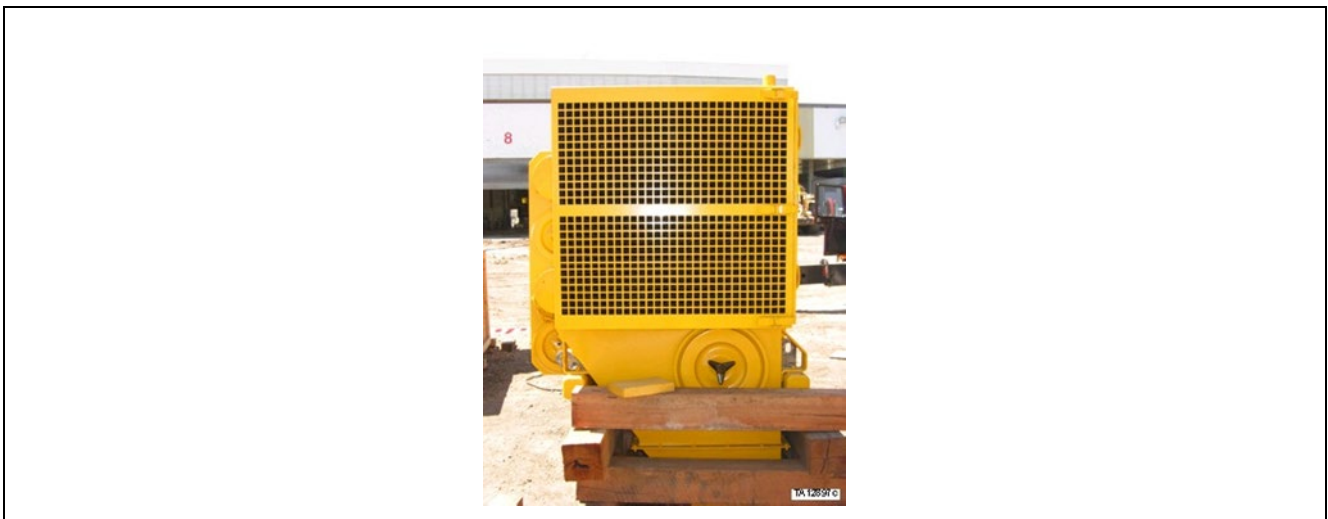
Figure 15. KLENZ™ and blower assembly supported by cribbing 3 of 3
