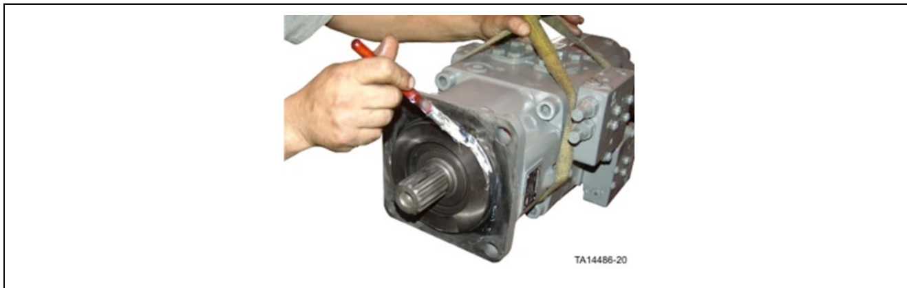
Figure 7. Application of assembly grease to pump O-ring and pump
