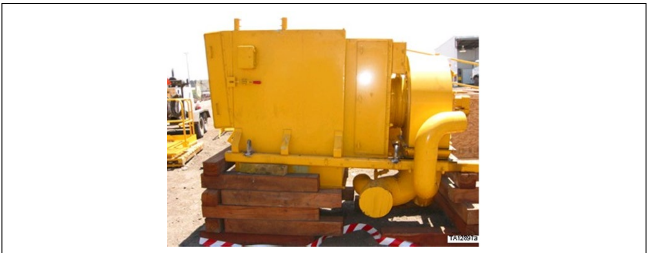
Figure 13. KLENZ™ and blower assembly supported by cribbing 1 of 3
