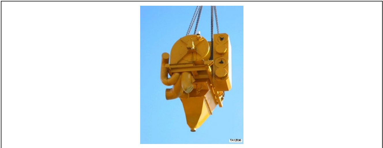
Figure 12. Hoisting of KLENZ™ and blower assembly
